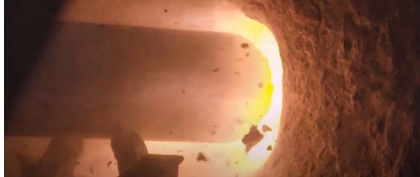
EarthGrid's plasma boring technology blasting through limestone. Photo from EarthGrid
